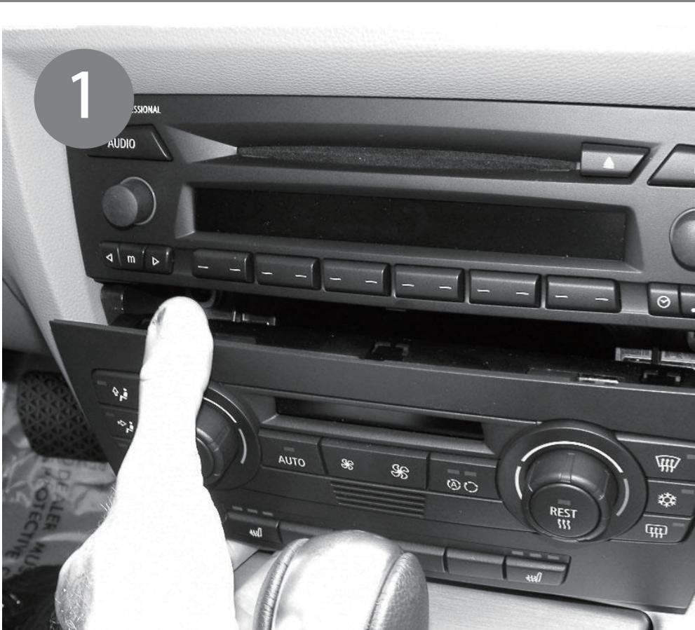
Carefully unclip and remove the climate controls.
