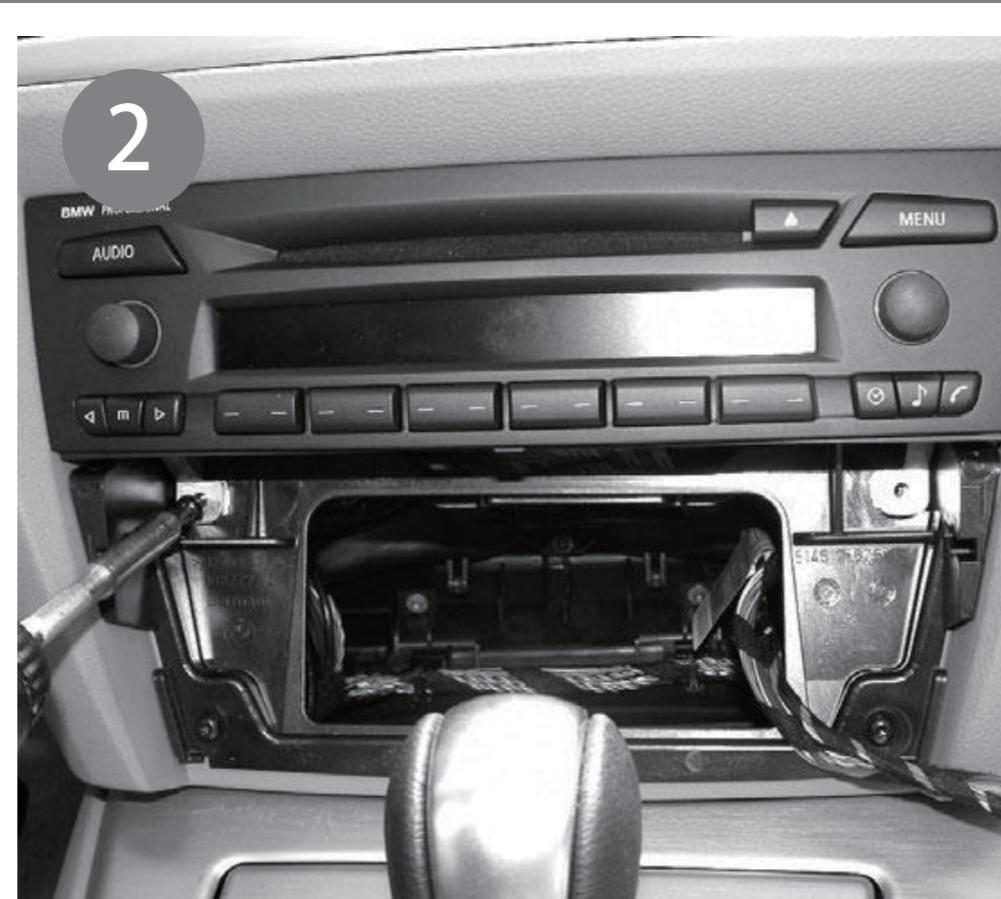
Remove two Phillips screws from the bottom of the radio
