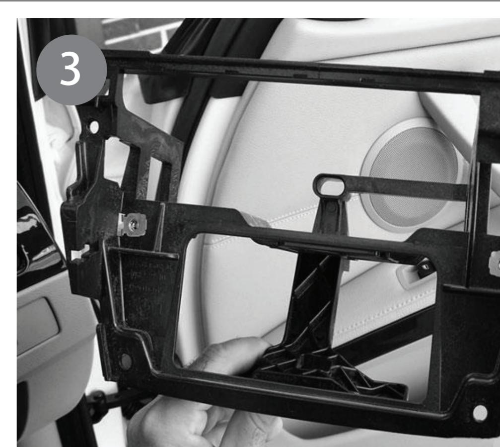
Remove the four Torx screws from the sub-dash bracket
