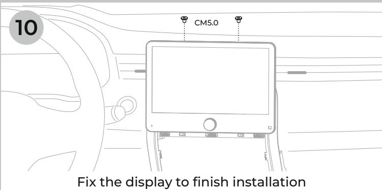
Fix the display to finish installation
