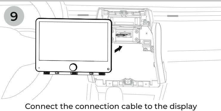
Connect the connection cable to the display
