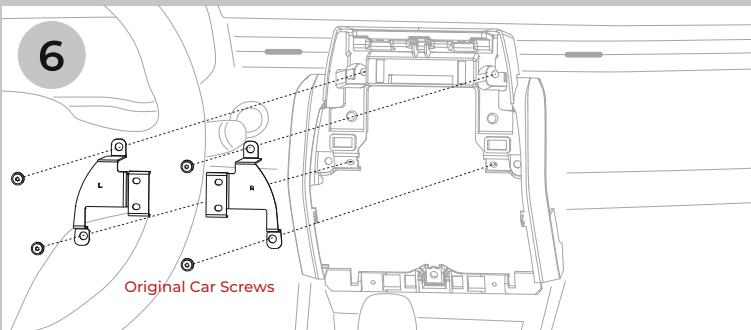
Put the mounting plates and the original bezel together
