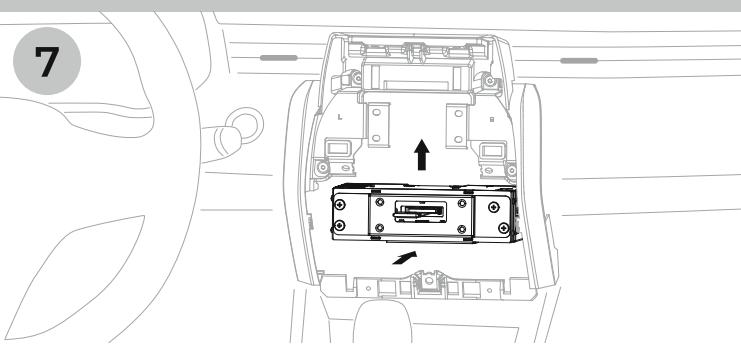
Put the main unit and the original bezel together
