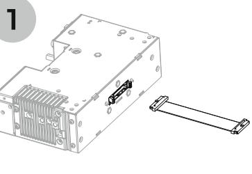
Connect the connection cable to the main unit
