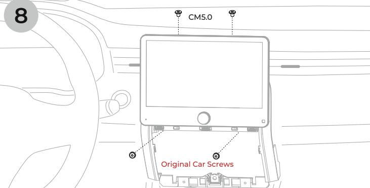
Fix the Dynavin radio to finish installation
