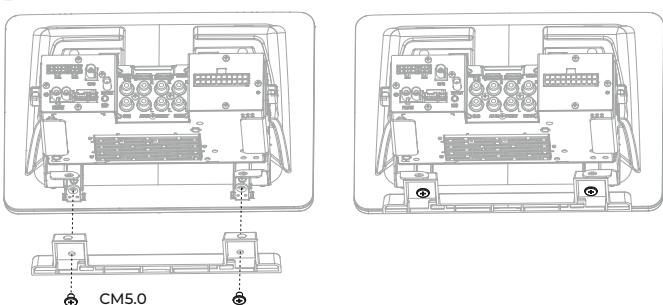
Put the mounting bracket and display together
