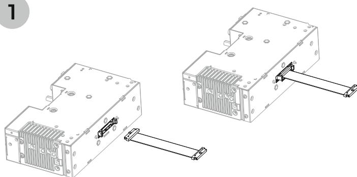
Connect the connection cable to the main unit
