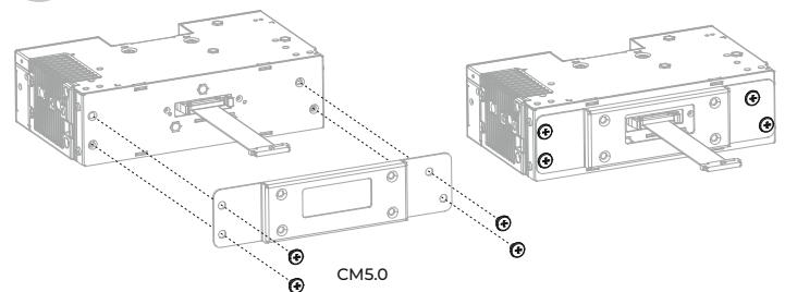
Put the main unit and the metal plate together
