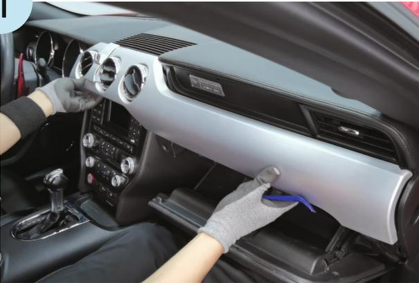
Removing the air conditioning panel
