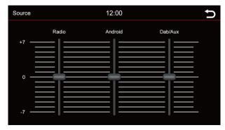
Here you can adjust the volume level of various sources. In the 0 range, the radio's set volume is used. In the range above or below 0, it is automatically adjusted by this level. Automatically adjusts by this level.
