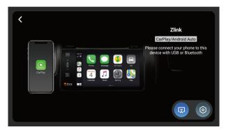
Before using wireless Apple CarPlay, turn on the BT function on your smartphone device Connect your smartphone to Dynavin unit via Bluetooth (Operation see page 19). After successful pairing, the device will automatically access the Apple CarPlay. Then you can control the smartphone via the Dynavin unit.
