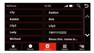
Use this menu option to bring up the contact list. As soon as you press a contact, a popup opens. The displayed contact with the stored phone number is called via the telephone key.
