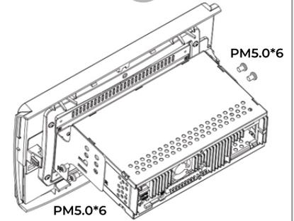
The screen mounting bracket has several options to allow the installer to adjust the chassis height position. Please use the chassis position that best suits the installation application.
