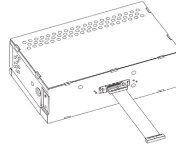
Connect the connection cable directly to the the headunit
