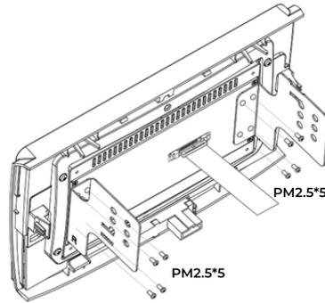
Attach the metal bracket on the panel with screws
