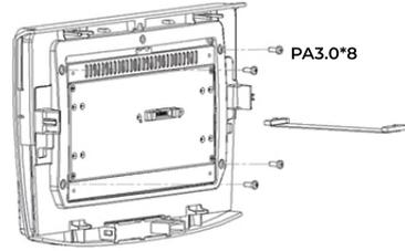
Attach the bezel on the panel with screws, then connect the connection cable directly to the panel
