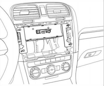
Attach the brackets with the original screws
