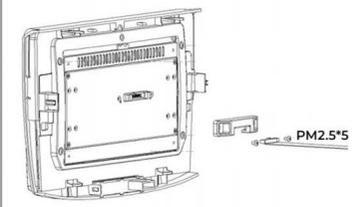
Attach the plastic bracket on the panel with screws
