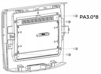
Attach the bezel on the panel with screws
