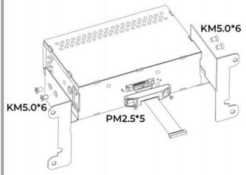
Attach the plastic bracket and metal bracket on the headunit with screws
