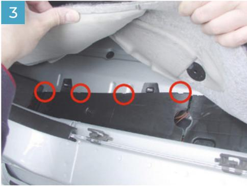
Raise the carpet and unhook the lid from the black plastic channel. The lid is hold with plastic hooks (marked).
