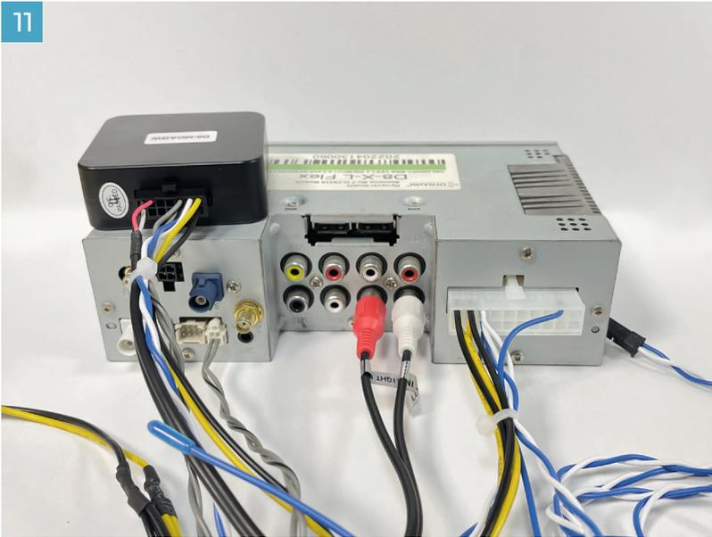
Connect the cable to the Dynavin unit as shown in the picture.
