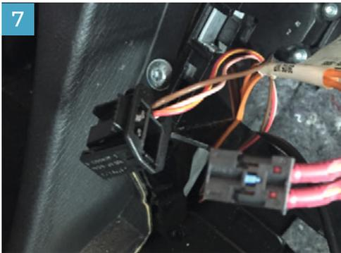
Pull out the MOST line from the original fibre optic cable.
