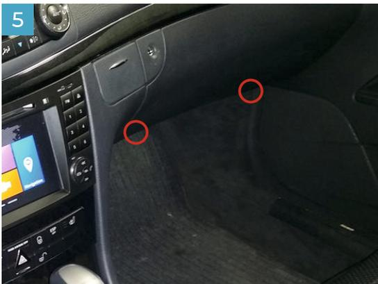
Remove the two marked screws (T20/T25) to remove the panel under the glovebox. The canbus distributor is placed on the left side.
