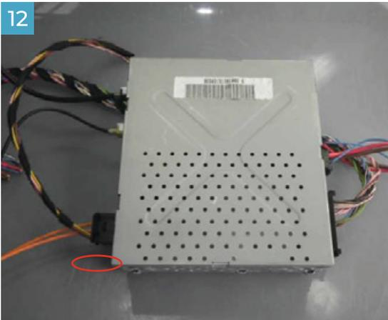
Pull out the radio antenna from the AGW (black connector).
