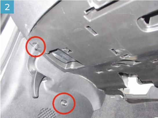
Remove the screws from the panel on the drivers side footwell with a torx screwdriver (2x T20/T25 Torx). One of the screws is placed in the middle, the other on the top. Carefully remove the plastic cap above the screw in the middle with a screwdriver or pocketknife. Pull out the sidepanel to the bottom left. It is anchored with other parts.
