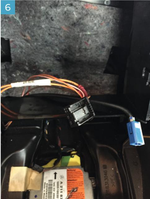
Picture shows original fibre optic cable.
