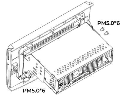
The screen mounting bracket has several options to allow the installer to adjust the chassis height position. Please use the chassis position that best suits the installation application.
