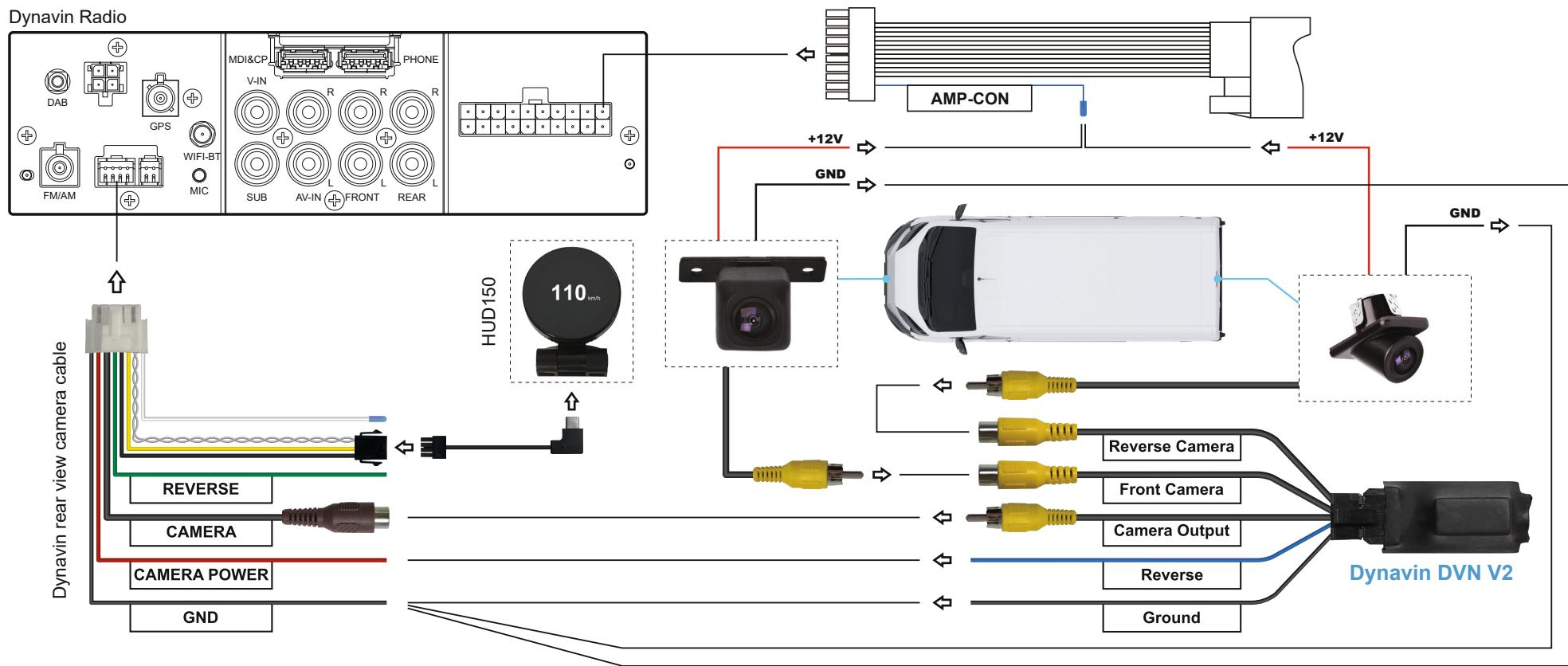
After the DVN-V2 is installed, you need to set it in the front camera setup menu and the Dynavin radio must be upgraded to the firmware after 2023-03.
